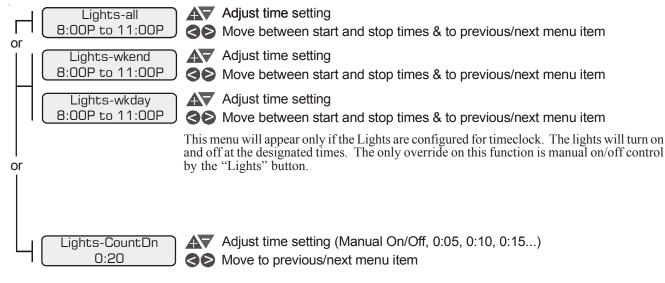
This menu will appear only if the Lights are configured for countdown timer. This setting is the time after you manually turn on the lights until the Aqua Logic automatically turns off the lights. You can also manually turn off the lights at an earlier time by pressing the LIGHTS button. If the Lights relay is on during the programmed off time, it may be because of freeze protection.
