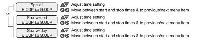
This menu is only available if the system has been setup for "spa only" or "pool and spa". During the programmed spa time, the Aqua Logic will turn on the filter pump and move the pool/spa valves into the "spa-only" position. The heater will automatically heat the spa up to the programmed spa temperature (page 7). This programmed spa operation will take precedence over all other automatic functions, only manual operation of the filter button or pool/spa valve button will override this function.
