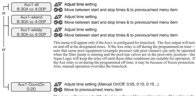
This menu will appear only if the Aux1 is configured for countdown timer. This setting is the time after you manually turn on the Aux relay until the Aqua Logic automatically turns off the relay. You can also manually turn off the relay at an earlier time by pressing the AUX1 button.
