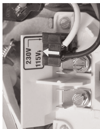
Figure 4B Voltage Change Plug Set for 115 Volts
